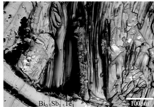
Fig. 10. Fracture surface of a \text{Bi}_{0.5}\text{Sb}_{1.5}\text{Te}_3/\text{Cu} joint soldered with Sn-3Ag-0.5Cu with an inserted sandwich structure of Sn-rich alloy thin films and a Ni barrier layer.
